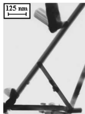
Figure 2. TEM image of the \alpha -AgBiS 2 nanowhiskers obtained from solvothermal process.
